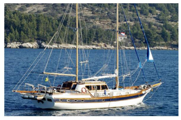
Typical ketch made by the masters of shipbuilding. The hull of the boat was made of grp and detailed project of its submarine part guarantee the maximal hardness and stability during the navigation. All interior and exterior coverings were made of the high quality mahogany and teak wood giving the warm and elegancy to this beautiful boat.
